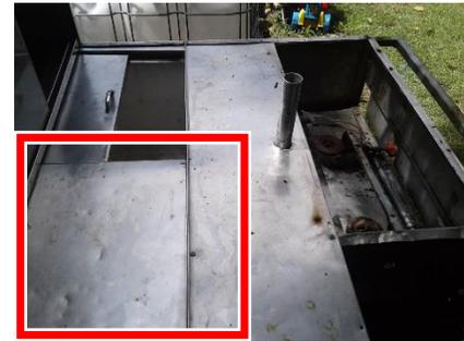
Go over the cart very carefully looking for dents, buckles and bends to the walls and shelving. Also get inside the cart cabinets looking for weld cracks or other signs of metal fatigue. Remember the cart is traveling on your city streets with only leaf springs to cushion the ride. Ever ride in the back of a pickup?
