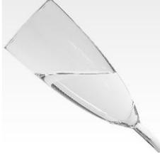
Pour some water into a clear cup and check for clarity. That is why you brought your own clear water. Debris in the water indicates a thorough cleaning of the water system is due.
