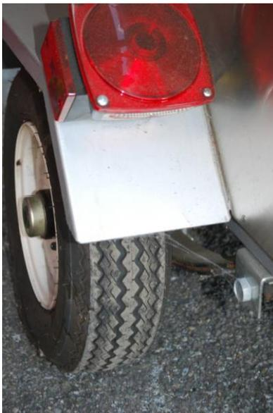
Plug the lights into a power source and verify all work as designed. Check the wiring for frays, brittle insulation and firm connections.
