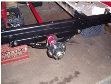
Using the flashlight look under the cart at the trailer and leaf spring assemble. Check for rust, corrosion and dirt.
